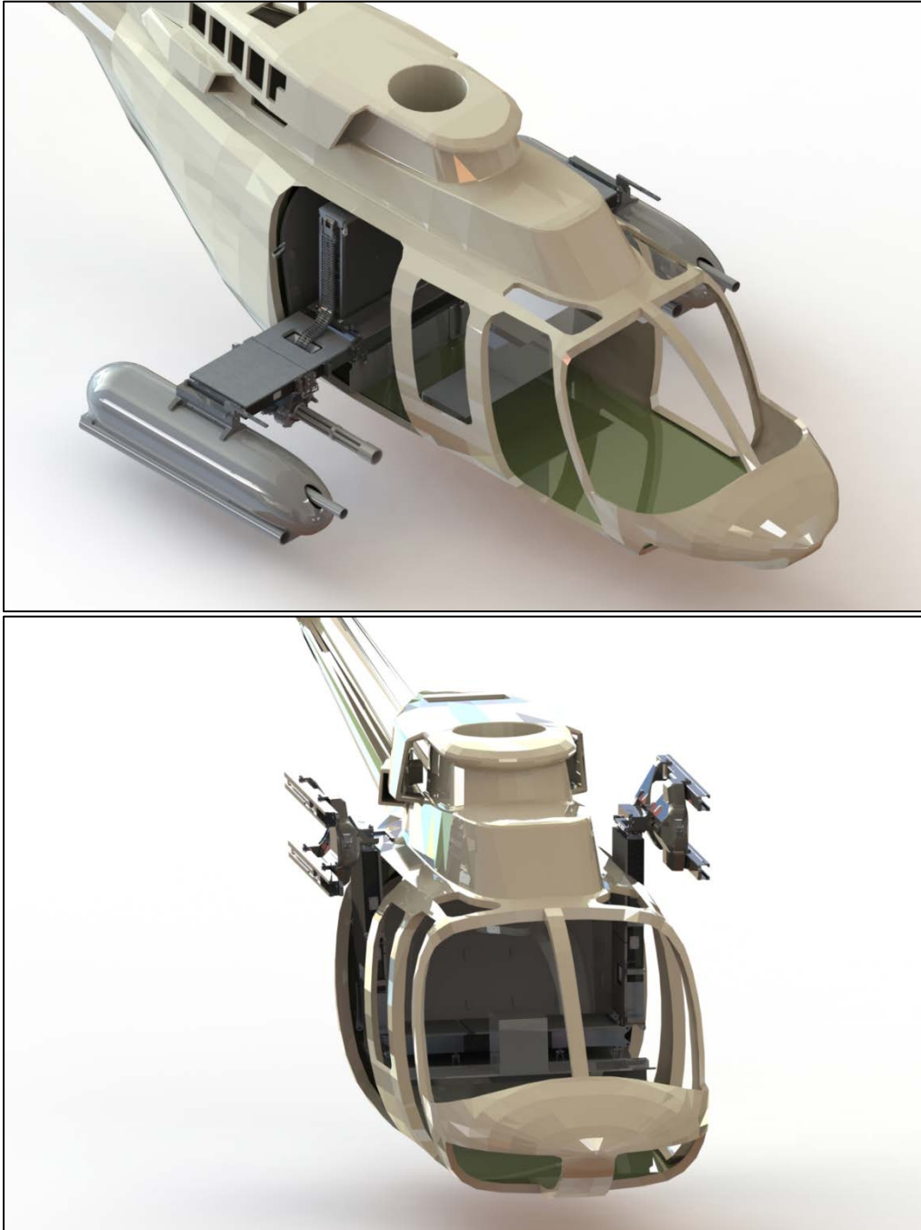
BELL 407 Series II COMPOSITE BASED Folding platform in aircraft shell
