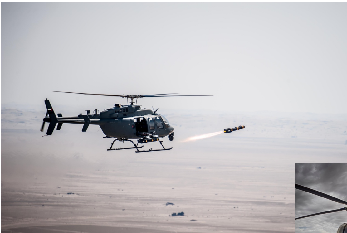
407 MRH firing Hellfire from the CAI Lightweight Missile Launcher
